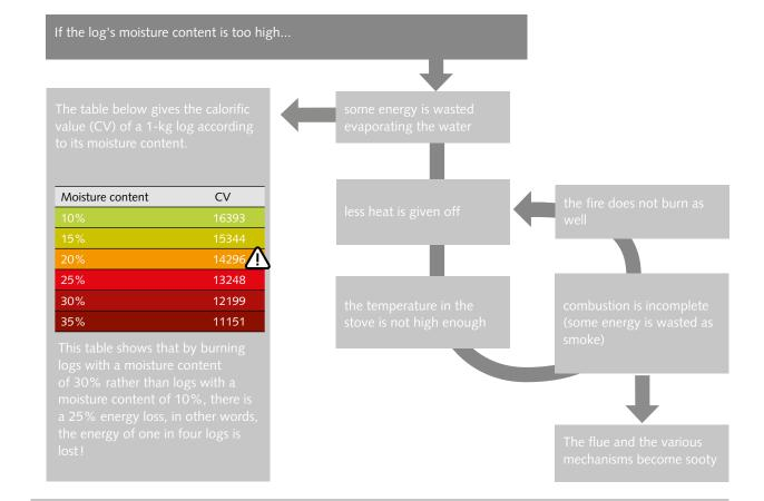
The vicious circle above illustrates the negative impact of a stove fuelled with wood that is too wet. By burning logs with a moisture content of 30% rather than logs with a moisture content of 10%, 25% of the log's energy is lost and an additional 25% is lost due to the poor operation of the stove.
