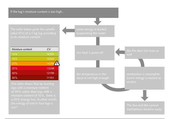
The vicious circle above illustrates the negative impact of a stove fuelled with wood that is too wet. By burning logs with a moisture content of 30% rather than logs with a moisture content of 10%, 25% of the log's energy is lost and an additional 25% is lost due to the poor operation of the stove.
